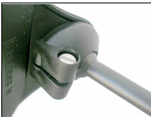
The ball-and-socket joint makes it easy to adjust, and if it gets wacked by a bollard, the mirror won't snap off. Smart Germans!
