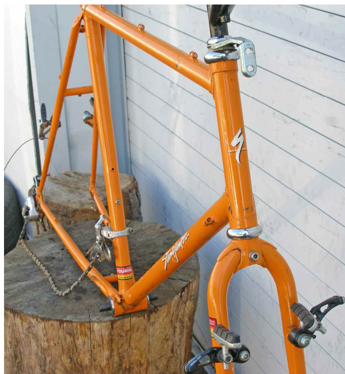
A rare lugged Specialized Stumpjumper with a rarer lugged uni-crown-style fork. Man, this is a nice old bike.
