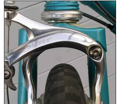
Good. You shouldn't have to look hard to see the air above the tire.
