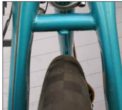
Good. Check fender (and tire) clearance everywhere the tire passes by the frame tubes. If it fits one place and not someplace else, you're stuck.
