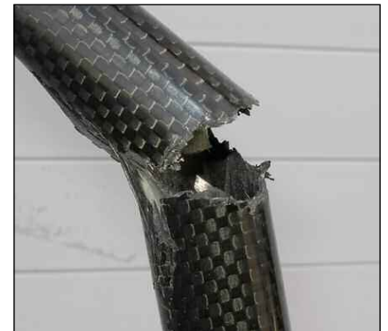
Bad. To be fair, this happened in an accident. But accidents happen, and a steel fork would have bent or dented, both of which are better than this.
