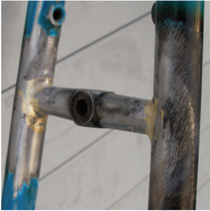
raised the brake bridge
