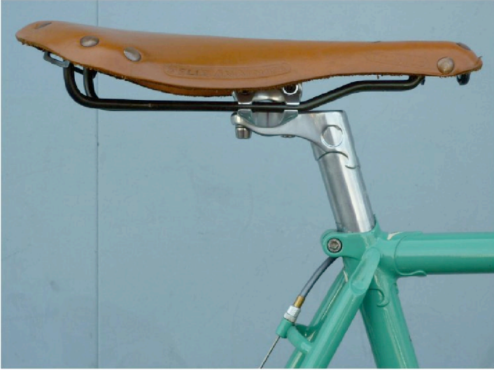
Lugged seat post and Selle Anatomica. Seat posts and saddles vary in how much you can shove the saddle back. This combo is the all-time champ.
