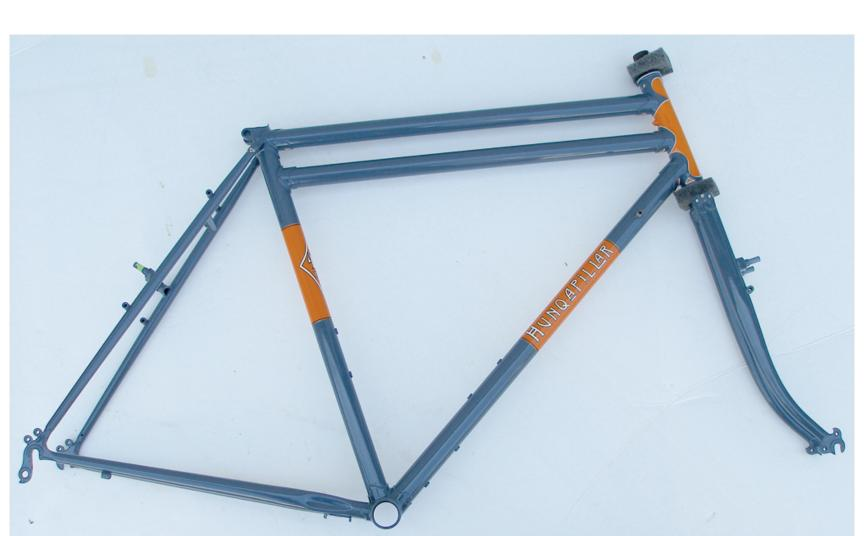
The 48 takes 26/559 wheels and has a single top tube. The 54 takes 700c wheel, with a single top tube (no room for two). The 58 (shown) and 62 take 700c and have doublers.
