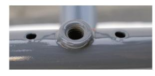
probably head lug lining, not sure. Kickstand plate is always a sure thing now on any non-Roadeo bike. Underside of brake bridge bossed & tapped for fendering.
