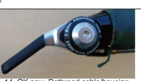
14. OK now. Rethread cable/housing, and rehook up the rear derailer.
