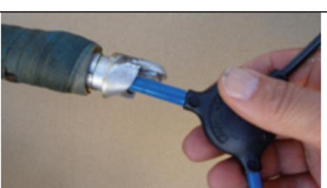
8. Loosen expanding bolt, extract pod.
