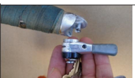
7. Pull off the shifter. Pull the shifter off.
