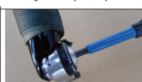
13. Use 4mm to tighten it on w/d'bolt.
